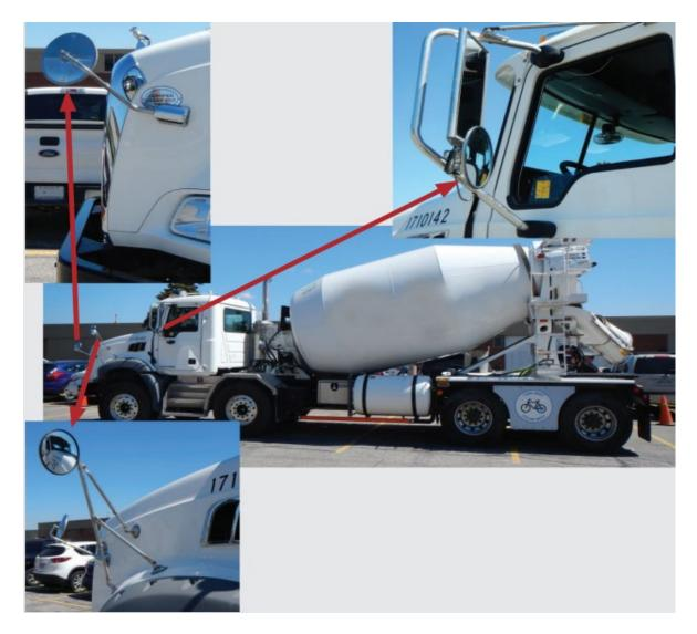
The goal of this mirror configuration is to adjust the mirrors so that objects can transition from one mirror field of-view to the next, thus allowing the Ready Mix driver to track the movement of vehicles and pedestrians around their truck
